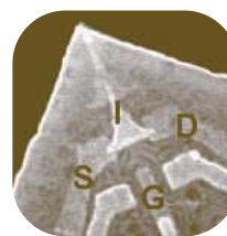
Cantilever-mounted single-electron transistor (D, drain; G, gate; S, source).
